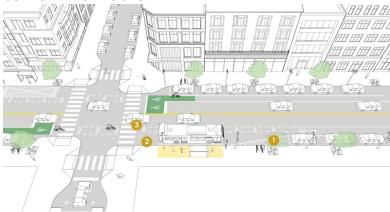
Innovation in road layout is a key aspect of reducing congestion. Curbside pull-outs allow buses to move out of the way of traffic. This allows for limited congestion as cars are not stopping behind the buses when they pick up or drop off passengers.
